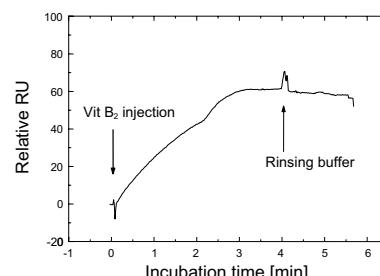
Figure 2: Surface plasmon resonance sensogram of vitamin B<sub>2</sub> binding to riboflavin binding protein after its photoimmobilization on an OptoDex® S modified gold platform.
